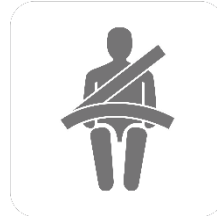
Safety Belt Not Fastened
